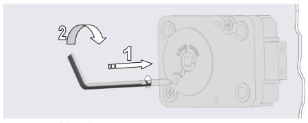
Fig. 2: Insertion of change key
